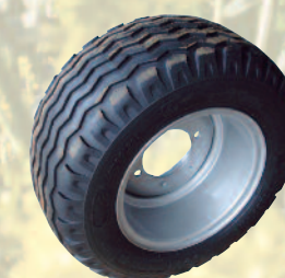
Wheel (Ø 777 mm, width 342 mm) with 340/55-16 tyres and 6 holes rim
