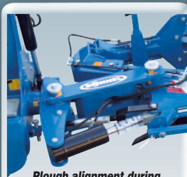
Plough alignment during turnover and mechanical adjustment of the first furrow
