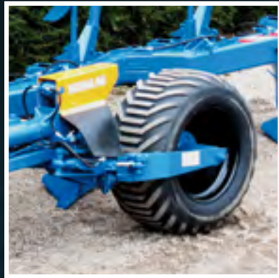
Large diameter directional wheel 500/45 - 22,5 with steering hydraulic cylinders.
