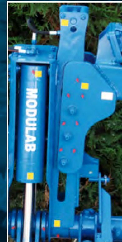
Hydraulic adjustment of the first furrow.
