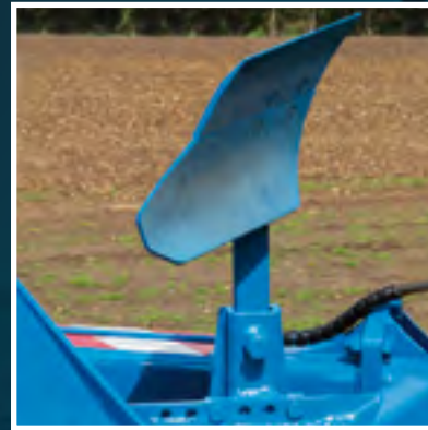
Adjustable skimmer in high and forward position.
