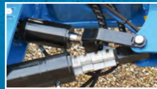
Hydraulic adjustment of the first furrow (optional).
