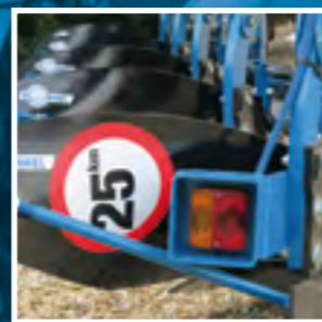
Integrated traffic lights.
